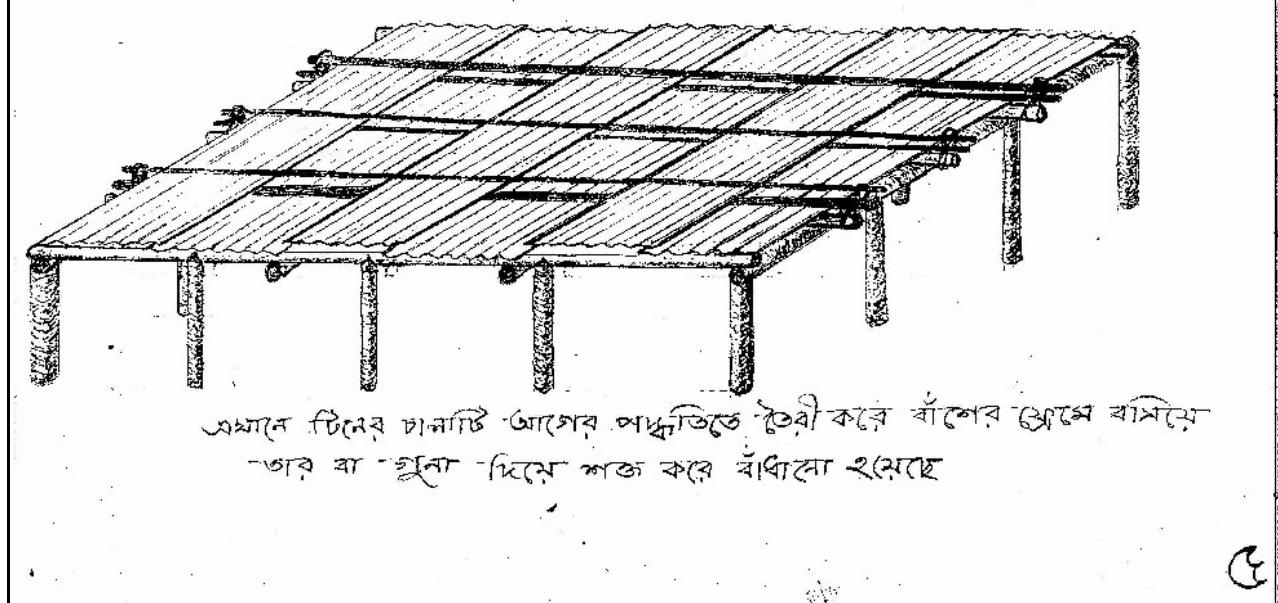
This is a bamboo frame which will be used on top of the CI Sheets.
